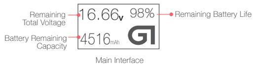
Note: When the battery is powered off, press the power button to check the battery life. (Main interface will display for 3 seconds while the LED Indicator light stays off during the whole process.)
