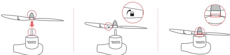
3. Attach the black nut propellers to the R motors in the same way.
